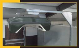
Electrical lifting unit for lifting the solarium. Including mounting kit, wall switch, electrical cable and connectorcable. Max. lifting weight 50 kg. Max. lifting height 1,5 mtr.
